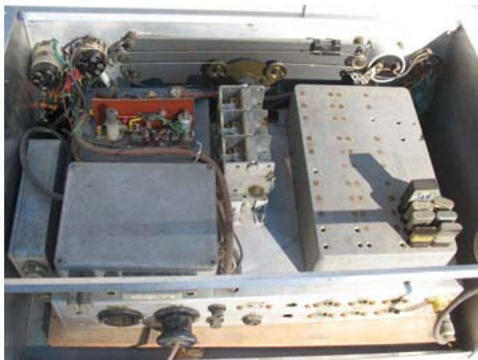
Rear view of the all-band receiver with the cover removed. Eddystone 898 slide-rule drive mechanism is visible at top. Two meter converter is above the diecast boxes, top left.
