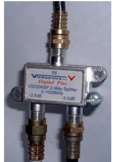
Two-way cable splitter provided in the OptimumOnline self-installation kit. Frequency range is 5-1000 MHz with each output port down 3.5dB compared to the input.
