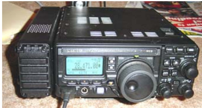
Yaesu FT-897 HF/VHF/UHF transceiver with FC-30 tuner attached and blue dial lights selected. (Photo by W2CH)
